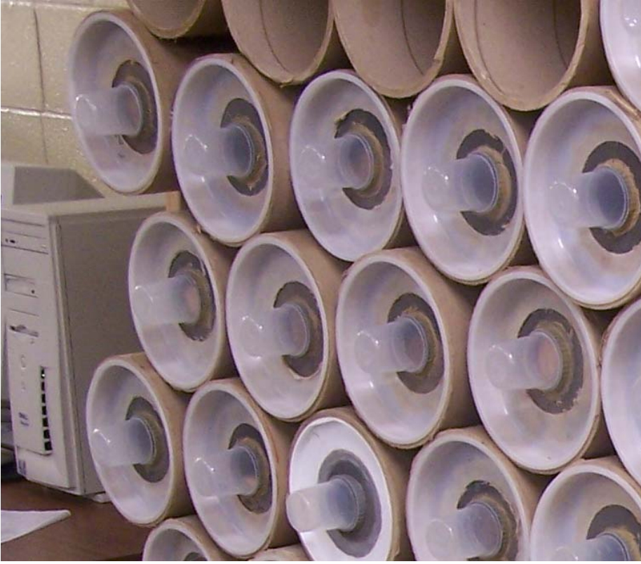
Photo 1. Cardboard rearing tube with collection cup for containment and collection of emerald ash borer adults in indoor treatments.
